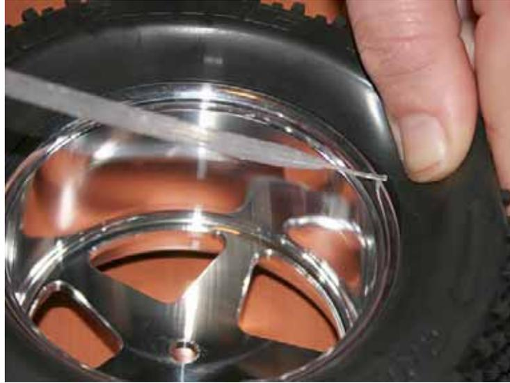
I find it's easiest to glue all of one side of the wheels and tires, and then start back over with the first one you did and glue the other side. This usually allows plenty of time for the glue to cure before you handle it again.
