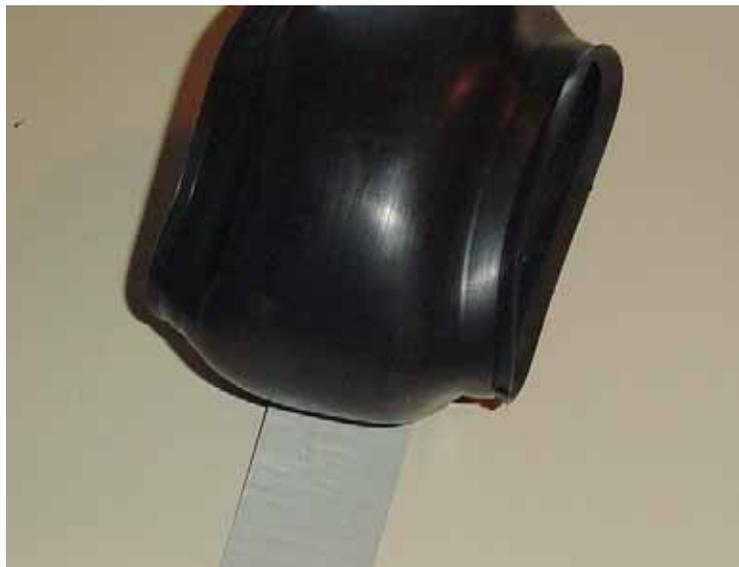
Allow the tape to overlap itself, and then make sure it's sealed well to the tire.
