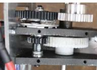
Kershaw's direct drive gearbox features a Traxxas Revo slipper unit and is designed for the Savage platform. The Stalwart V3.1 uses an improved version that encloses the gears. My experience with this gearbox has been great. It provides solid performance and so far has been bulletproof.
